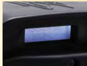
LCD monitor Displays the current date, time, latitude and longitude. The display mode is easily switched by a button.
